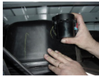
Step 3: Slide fuel valve from bracket.
